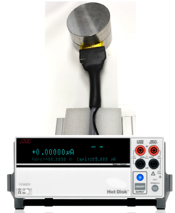
Hot Disk M100 for K-value Test Applicable range 0.03-40 W/mK
